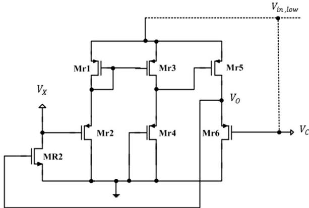
**Fig. 5** The voltage controlled grounded resistor circuit
