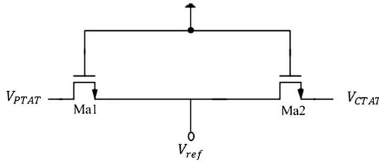
**Fig. 3** The voltage averaging circuit
