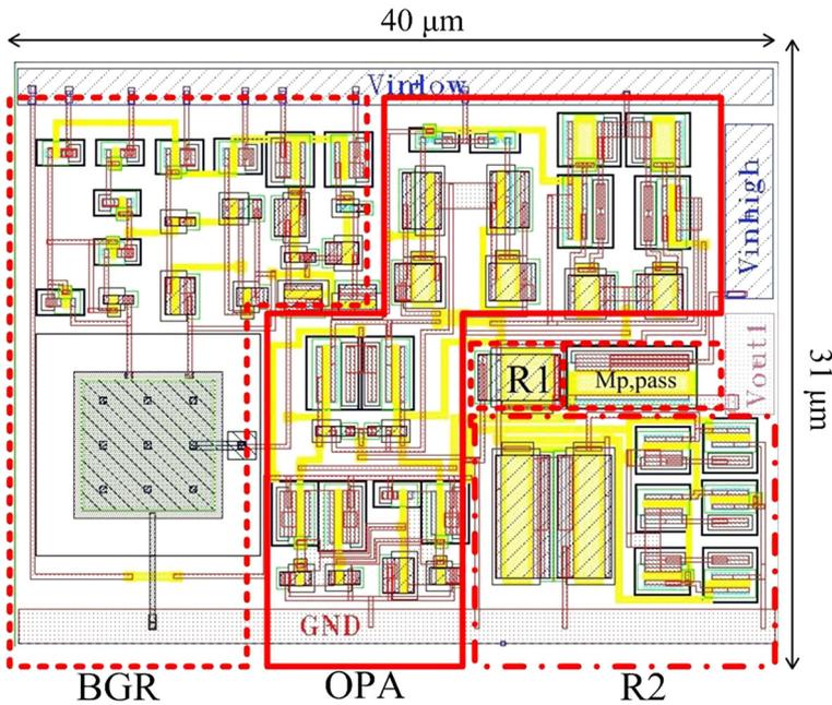
**Fig. 11** The layout of the complete proposed voltage regulator
