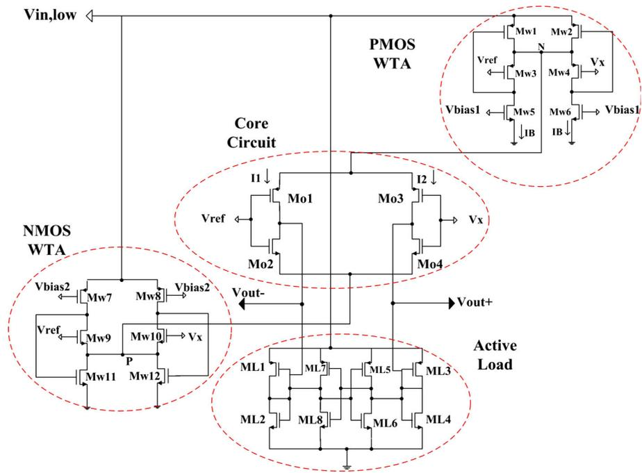
Fig. 4 The complete proposed OPA circuit
