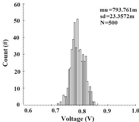
Fig. 10 The regulator output of the Monte Carlo simulation for the process variation and mismatch
