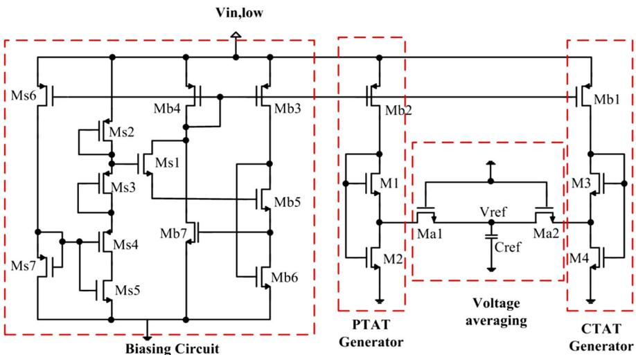
Fig. 2 The proposed reference voltage circuit [7]
