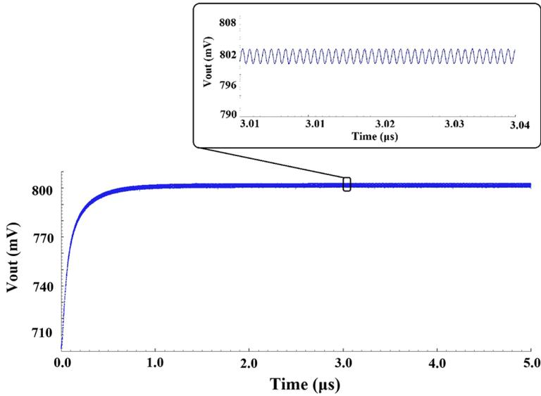
Fig. 9 The optimized regulator output voltage
